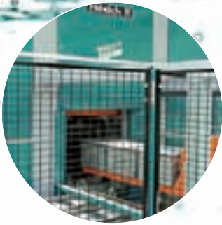
Fully automatic loading by multi-tracked roller conveyor
