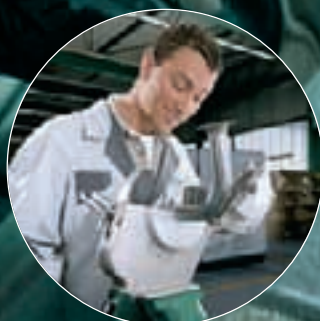
Orbital welding device for optimal smooth welding seams even in the pipes interior.
