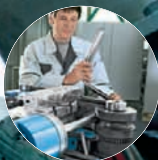
CNC pipe bending machine for pre-assembling stainless steel pipe lines
